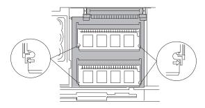
While holding the strap  $\blacksquare$  , pull the DIMM adapter toward the front to remove it.
